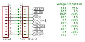
All pins of the connectors potentially carry 24V => cannot directly feed into Arduino!
